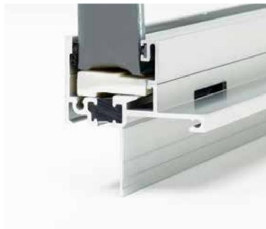
Milgard Thermally Improved Aluminum windows consist of extruded aluminum, where a “channel” is cut through the aluminum and polyurethane is poured into this channel to separate the interior from exterior extrusion. This process is done to reduce thermal transfer and improve energy efficiency.
